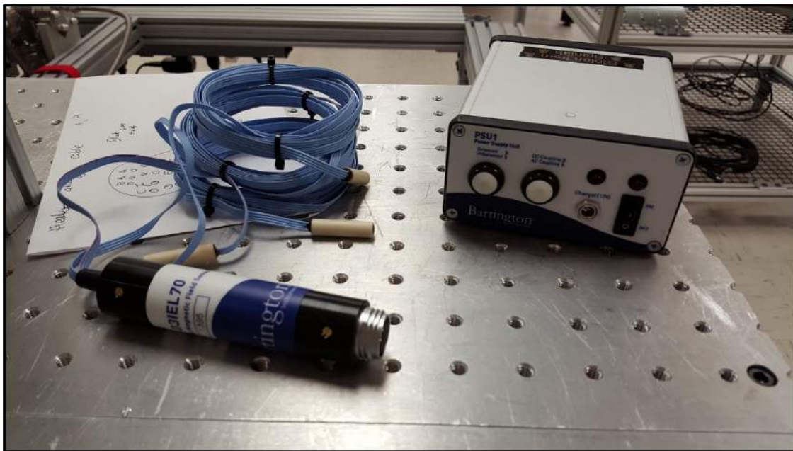
Figure D3: Fluxgate: Bartington Mag03IEL70. 16 kHz excitation frequency, noise floor is 6 \text{ pT}_{\text{rms}}/\sqrt{\text{Hz}} . Power supply: Bartington PSU1. 5 \text{ pT}_{\text{rms}}/\sqrt{\text{Hz}} noise floor. Data acquisition: NI PCie-6320. 16-bit. 2 mV noise floor on 10 V scale.
