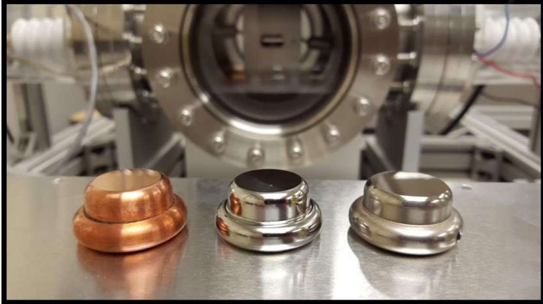
Figure 3.2: From left to right: a copper, niobium, and titanium electrode.
